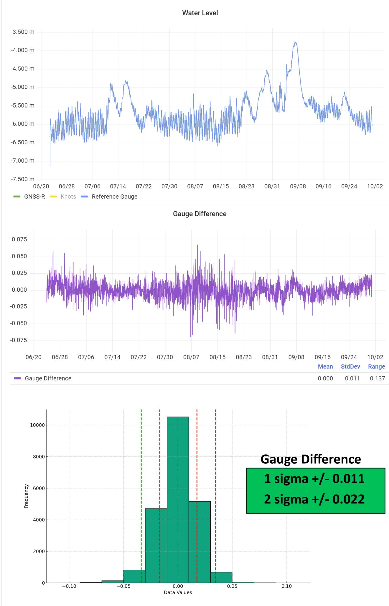
A Septentrio Mosaic Go and a bubbler/pressure based water level sensor were installed on the left bank of the river at Buckland, Alaska for 3 summer months. The river has a tide signal but is also affected by upstream influences and experienced multiple high water events. The site shows the technique can successfully capture irregular water level variations on a river. The large footprint, calm water, and the three meter bank produced excellent results.
